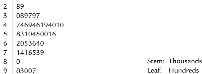
FIGURE 3.13 Stem-and-leaf display of the average tuition and fees data using truncated stems.
